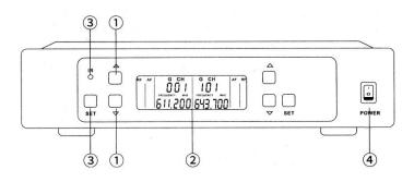
(1) Function Buttons: Used for channel selection, frequency adjustment/synchronization/scanning, etc.
